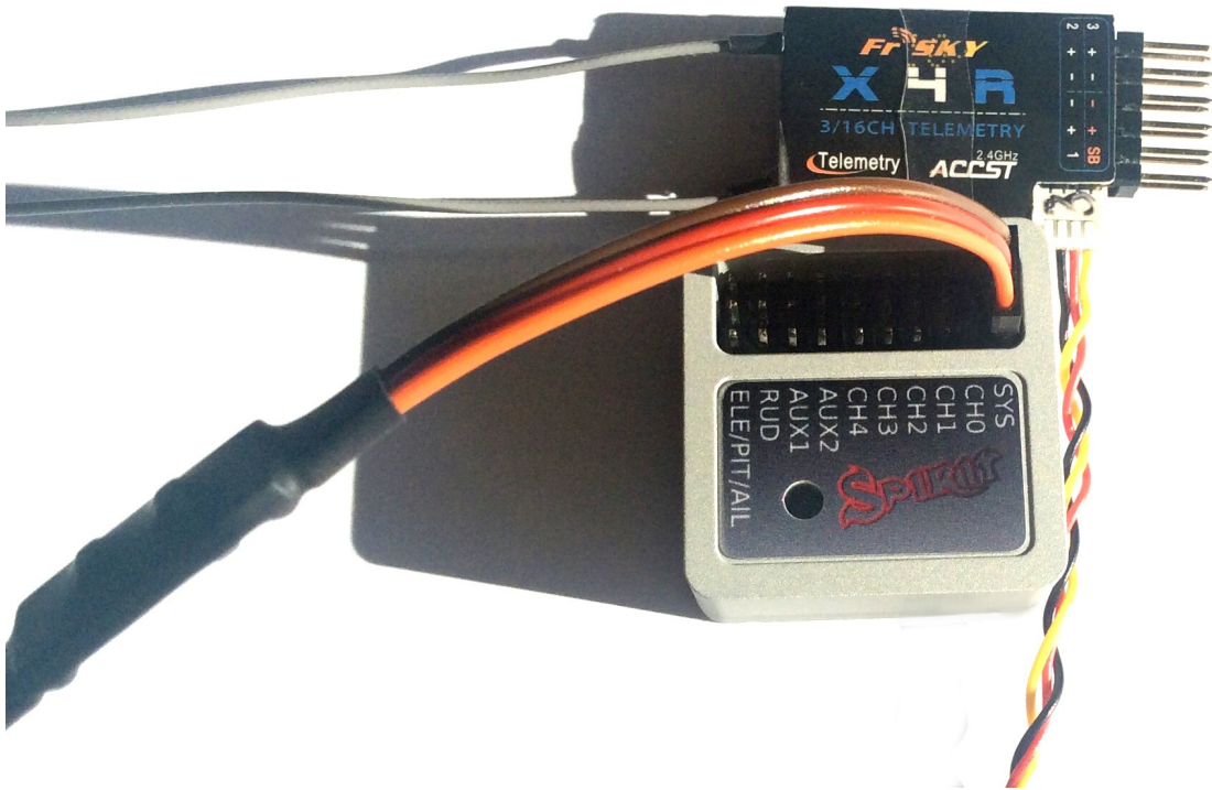
Example 1: connection scheme for the Integration part with X4R-SB receiver
